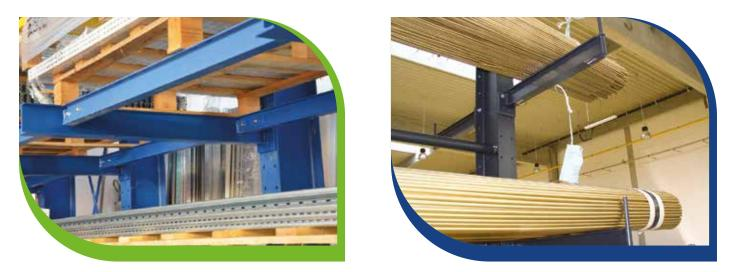
Cantilever racks can be used not only for storing materials of big dimensions, such as bars, oversized pallets, etc., but it is also used by customers with different types and sizes of pallets that are inappropriate for storage on a pallet rack.
